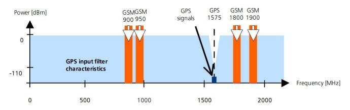
ST310Aconfigured SAW to reduce the out-band jamming by adding SAW filter.
